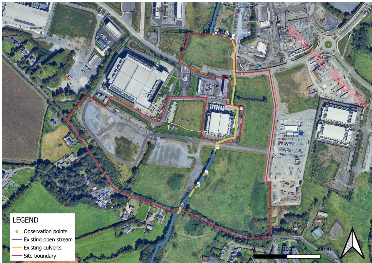
Figure 1.12: RHAT observation points for the on-site watercourse traversing the Proposed Development (points 1-4) and the off-site watercourse downstream of the Proposed Development (points 5-7).
